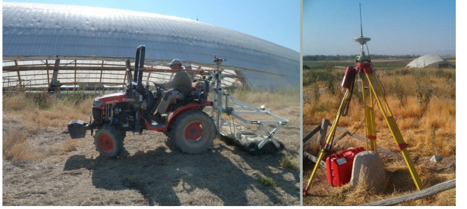
Left, the STREAM X GPR survey was completed with a tractor for pulling the system. Right, the Leica Viva GPS base station set up on the East Mound.
