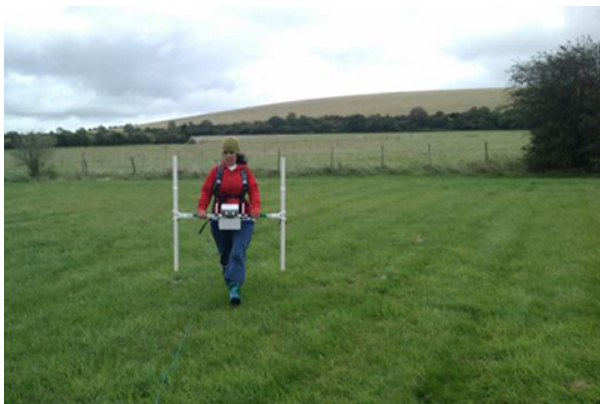
Figure 7.2. Magnetometer survey being conducted using a Bartington Instruments Grad 601 dual sensor fluxgate gradiometer.
