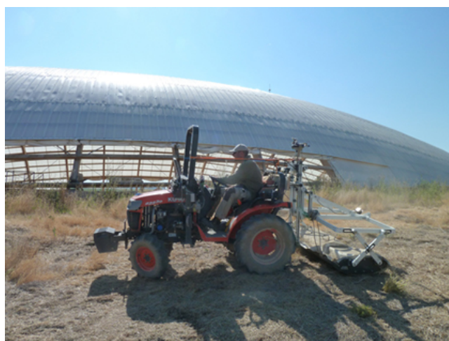
Figure 7.3. The STREAM X GPR survey being conducted, using a tractor for pulling the system.
