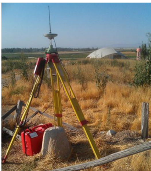
Figure 7.1. The Leica Viva GPS base station set up on the east mound.
